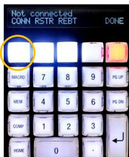
CONN (Connect) – The LCD lists detected systems or “Not Connect”
